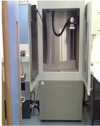
Figure 3.2: The X-Rays cabinet XRAD 225
