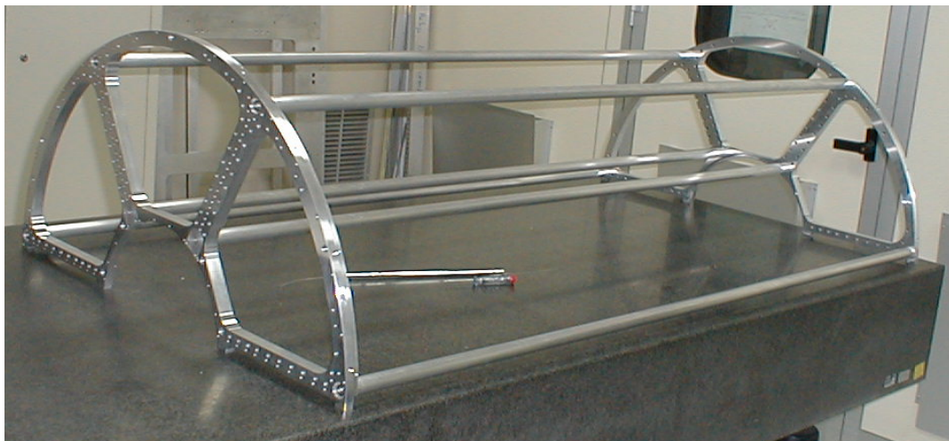
Figure 2.10: A full size prototype of the foreseen mechanical frame to support one half of the tracker. Design and construction by D.Orecchini (SSE-LNF, Frascati).
