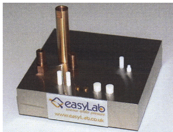
Figure 8.5: Mcell components and mounting platform.
