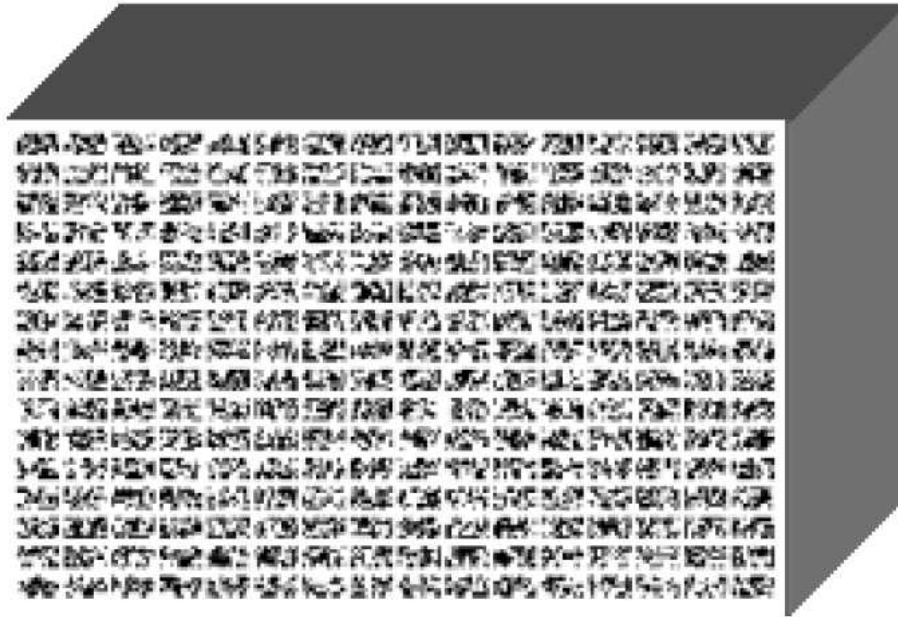
Figure 4.5: Representation of a Detector Plane Histogram (DPH). It is three dimensional in the sense that there are two spatial dimension (that of the detector plane) and one spectral dimension.
