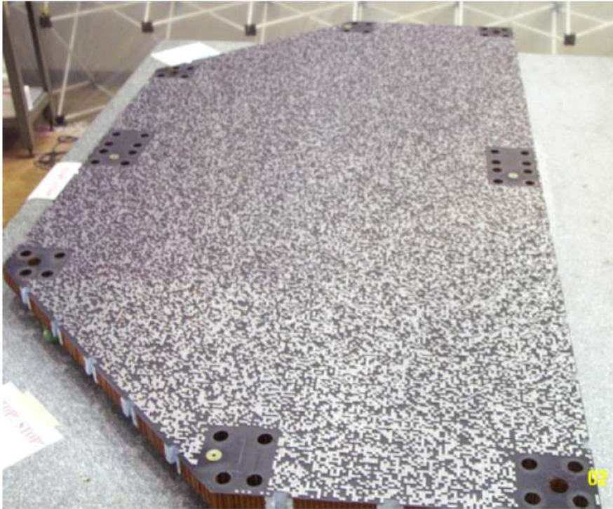
Figure 4.3: Picture of the BAT coded aperture mask before Swift launch.
