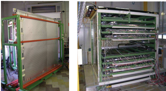
Figure 3.2: Left: RPC chambers just arrived from GT in Pavia site. Right: test cosmic ray telescope with five RPCs under test inside.
