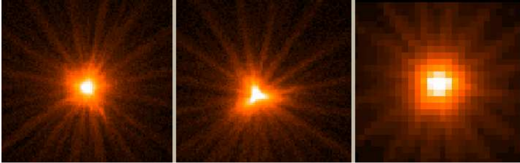
Figure A.2: On axis point spread function of the MOS1, MOS2 and pn X-ray telescopes (left to right) registered on the same source with each MOS camera in Small Window Mode, and the pn camera in Large Window mode. The pixel size is 1.1 arcsec square for the MOS, and 4.1 arcsec square for the pn. A square root scale has been used to visualize the wings of the point spread function. The core of the PSF is piled-up for this source, with a different factor for the MOS and the pn. The star-like pattern is created by the spider which supports the 58 co-axial Wolter I mirrors of the telescope. The shape of the point spread function core is slightly different for all cameras, with MOS2 having a somewhat triangular shape.
