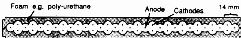
Figure 3: Cross section of a 23 cm wide multicell unit with 16 wall-less drift cells. The single wires are anodes, the pairs of wires shown are cathodes and serve as separation between two cells.
